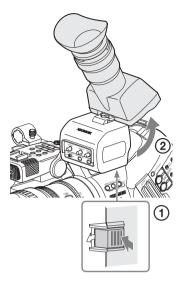
Normally use it in the locked position. Although you can open it farther from the lock position, once return it to the closed position to lock it at the 120-degree position again.
